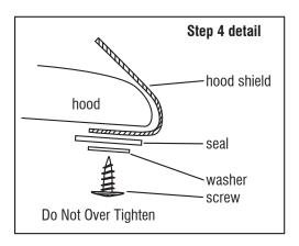
**IMPORTANT:** Before driving, ensure the hood shield is properly secured to vehicle. Clean with a **SOFT** cloth and soap and water ONLY! Using abrasive cleaners, chemicals, or solvents will **VOID** the warranty on this product.
